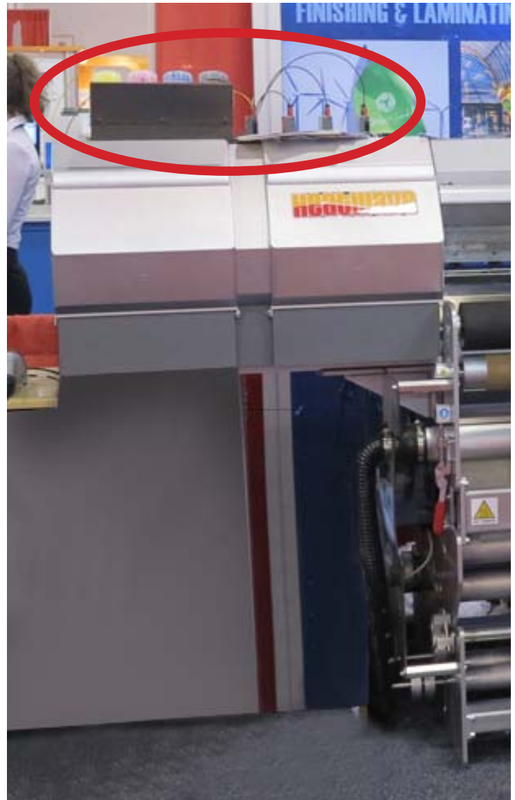
Ink system at the back side of the printer.
