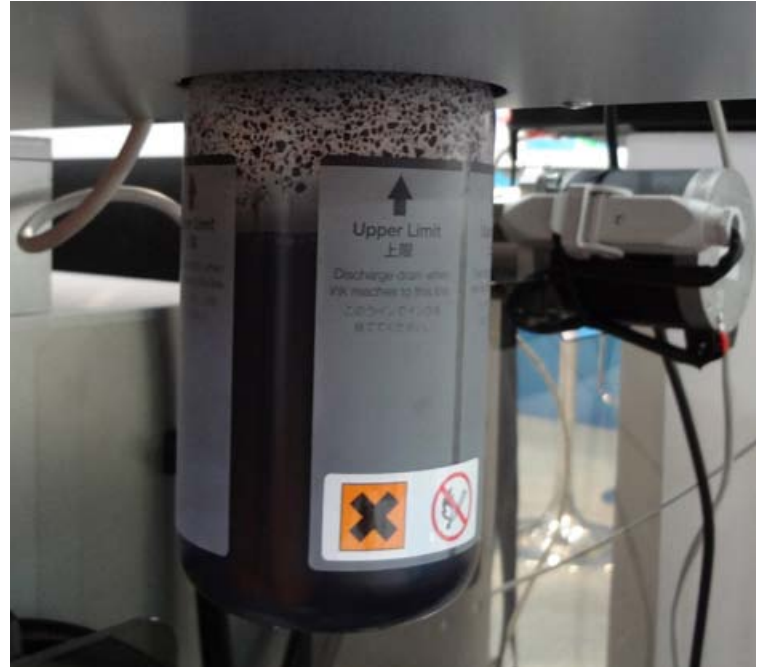
Ink waste bottle located below the printer chassis.
