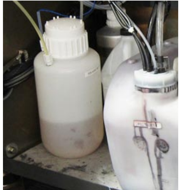
The solvent container is located in the rear cabinet, next to the waste ink tank.
