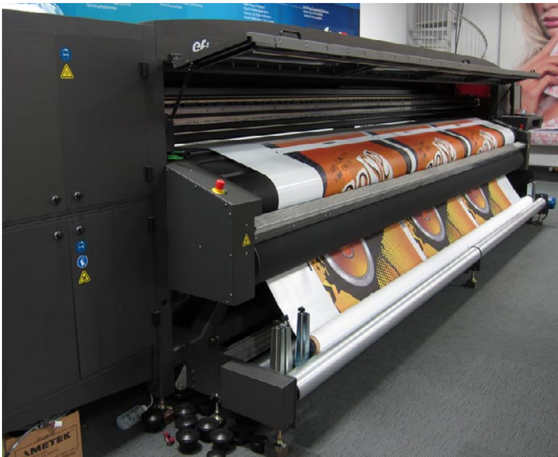
A front view of the media path. As you can see there is no dancer bar at the front. Once media is passed through the pinch rolls, it goes straight to the core.
