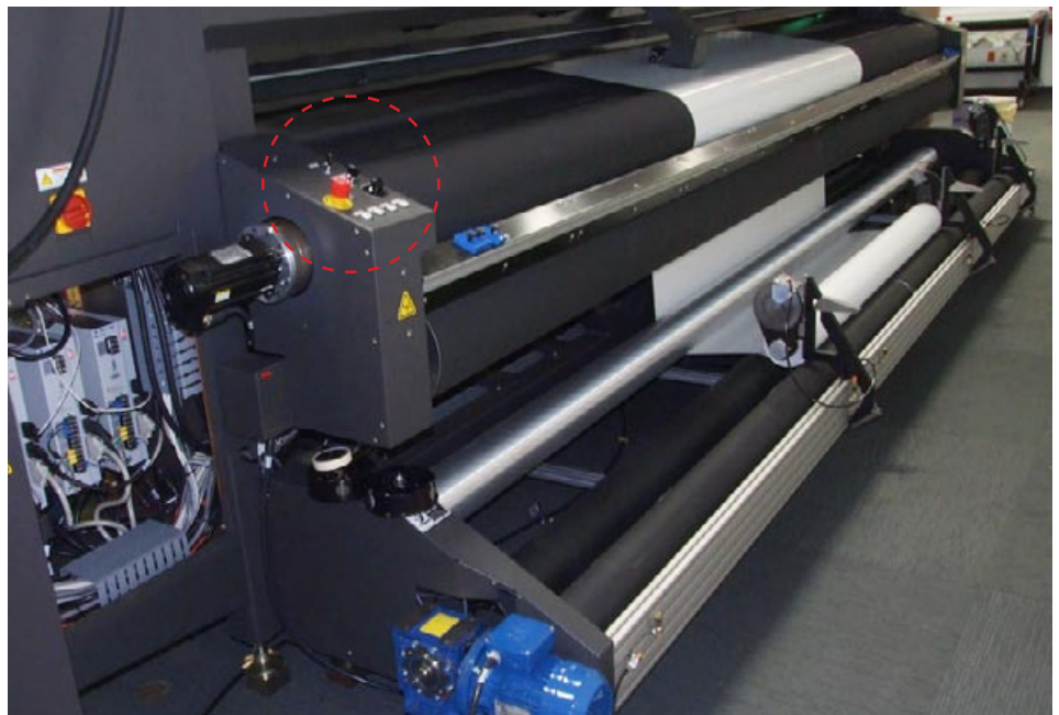
Since most operations are performed via software, you find only a few buttons at the back.
