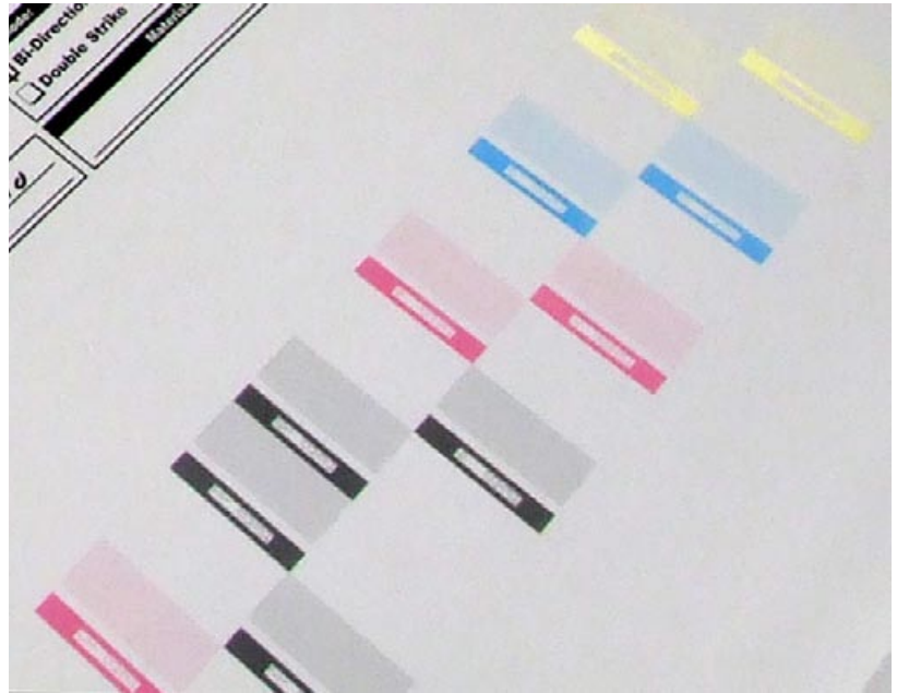
Nozzle test pattern. Absent or interrupted lines in this pattern are the sign that a nozzle is blocked.
