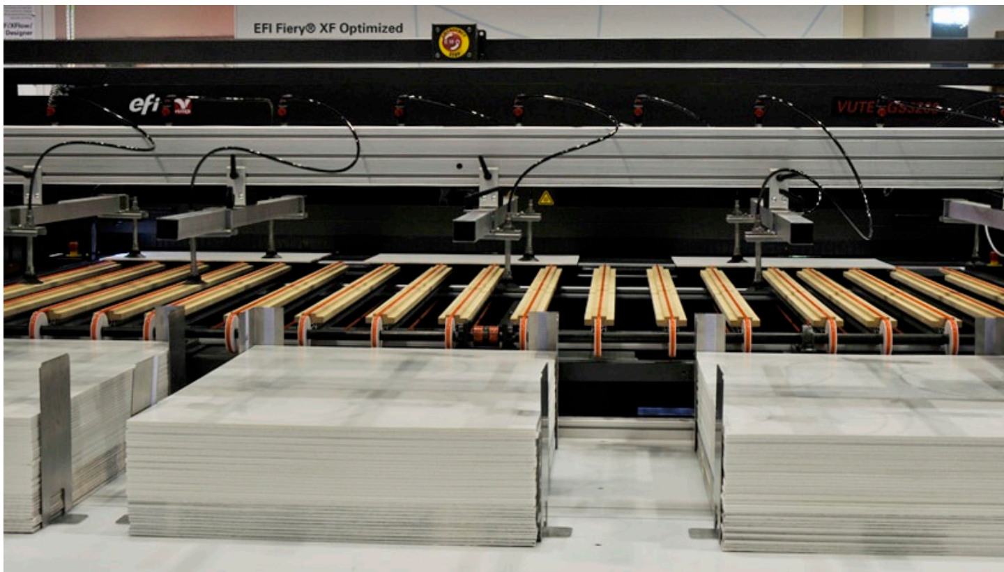
Media is stacked at the back. Metal stops keep the pile from moving.
