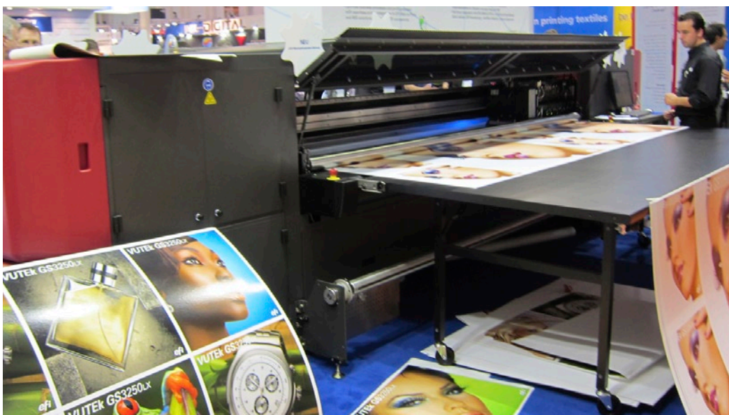
EFI VUTEK GS3250 LX printer launched at FESPA 2011. The light inside the printer is blue because this model has LED technology UV lamps.
