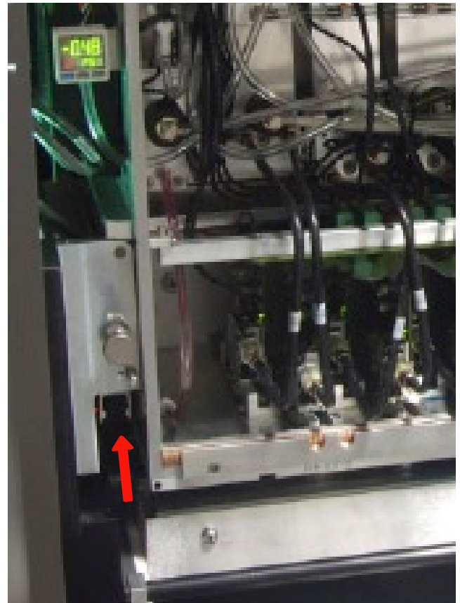
There is one static dissipater bar at each side of the printhead carriage.
