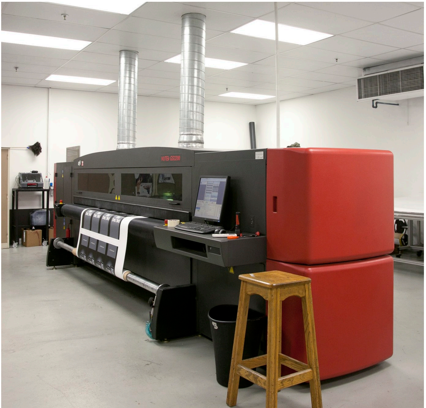
The EFI VUTEK GS3200 printer at ARTONE Press. You can see the two exhaust pipes on top.
