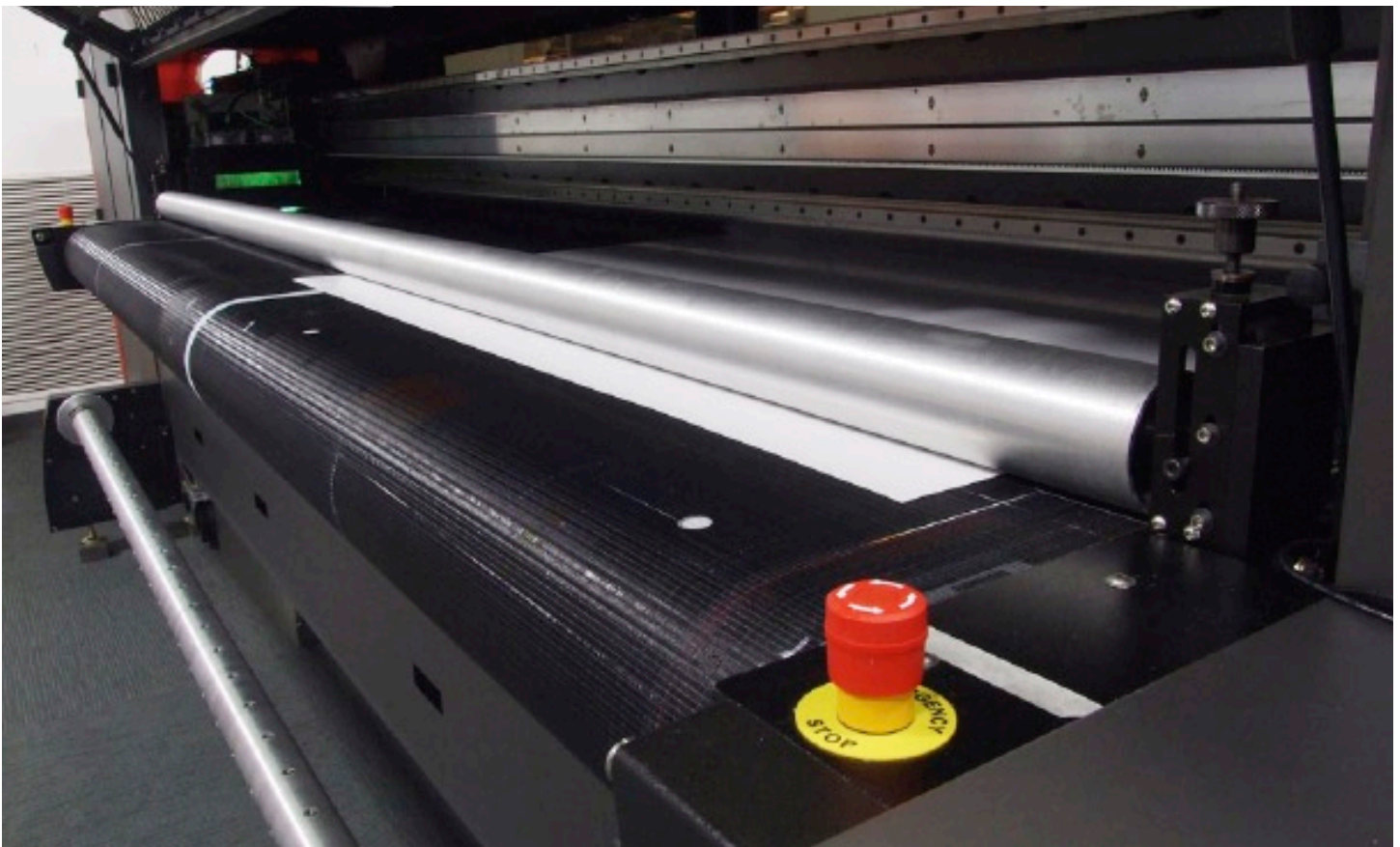
The transport belt can be moved forwards or backwards.
