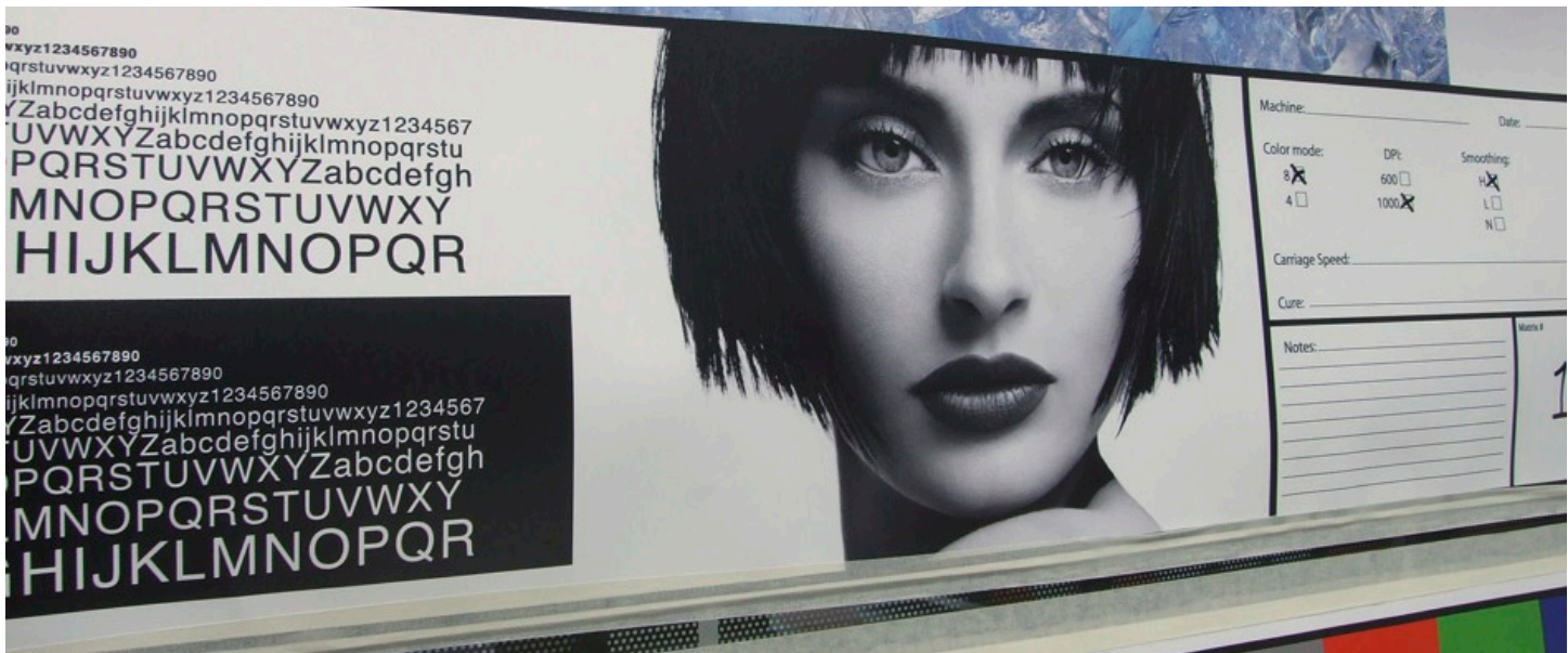
Small text is tested with black over white background and white over black background to see the different results.
