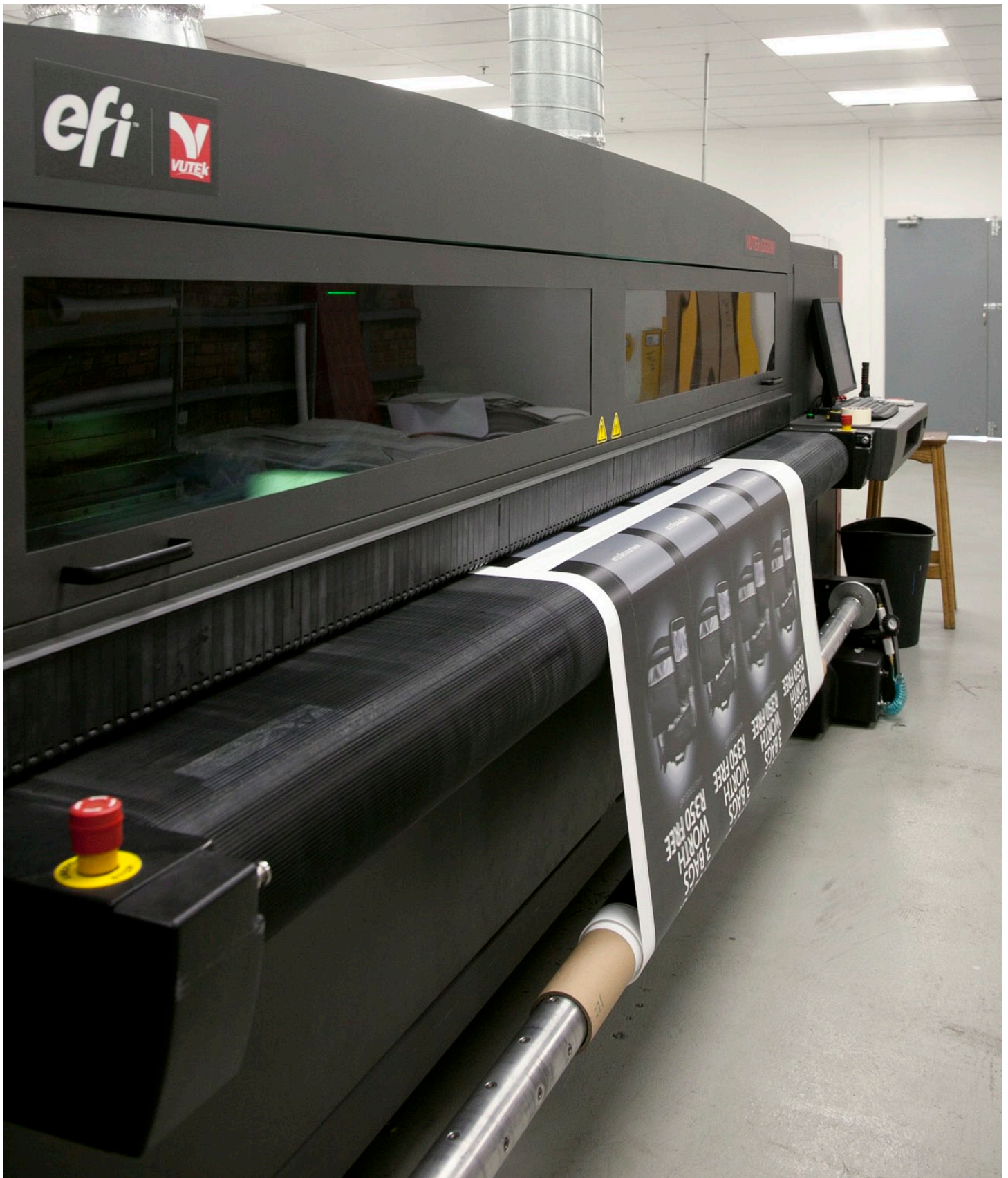
EFI VUTEK GS 3200 at ARTONE Press, a sign shop in Johannesburg, South Africa. The advantage of a combo printer (based on a transport belt) is the ability to print on both rigid and roll media.
