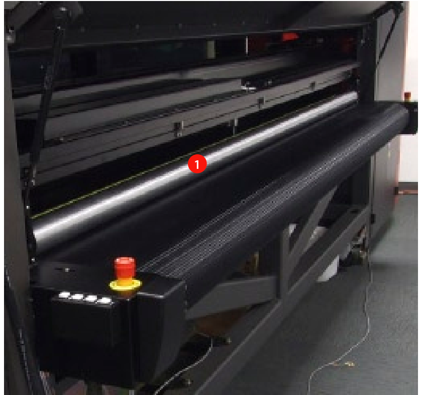
The hold down media roller (1) helps the system to keep media flat.
