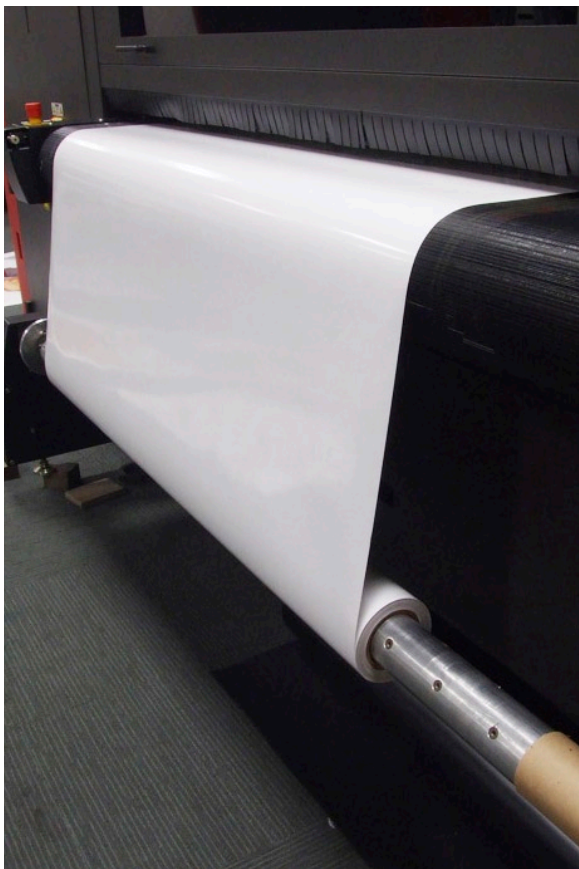
The hold down media roller (1) helps the system to keep media flat.
