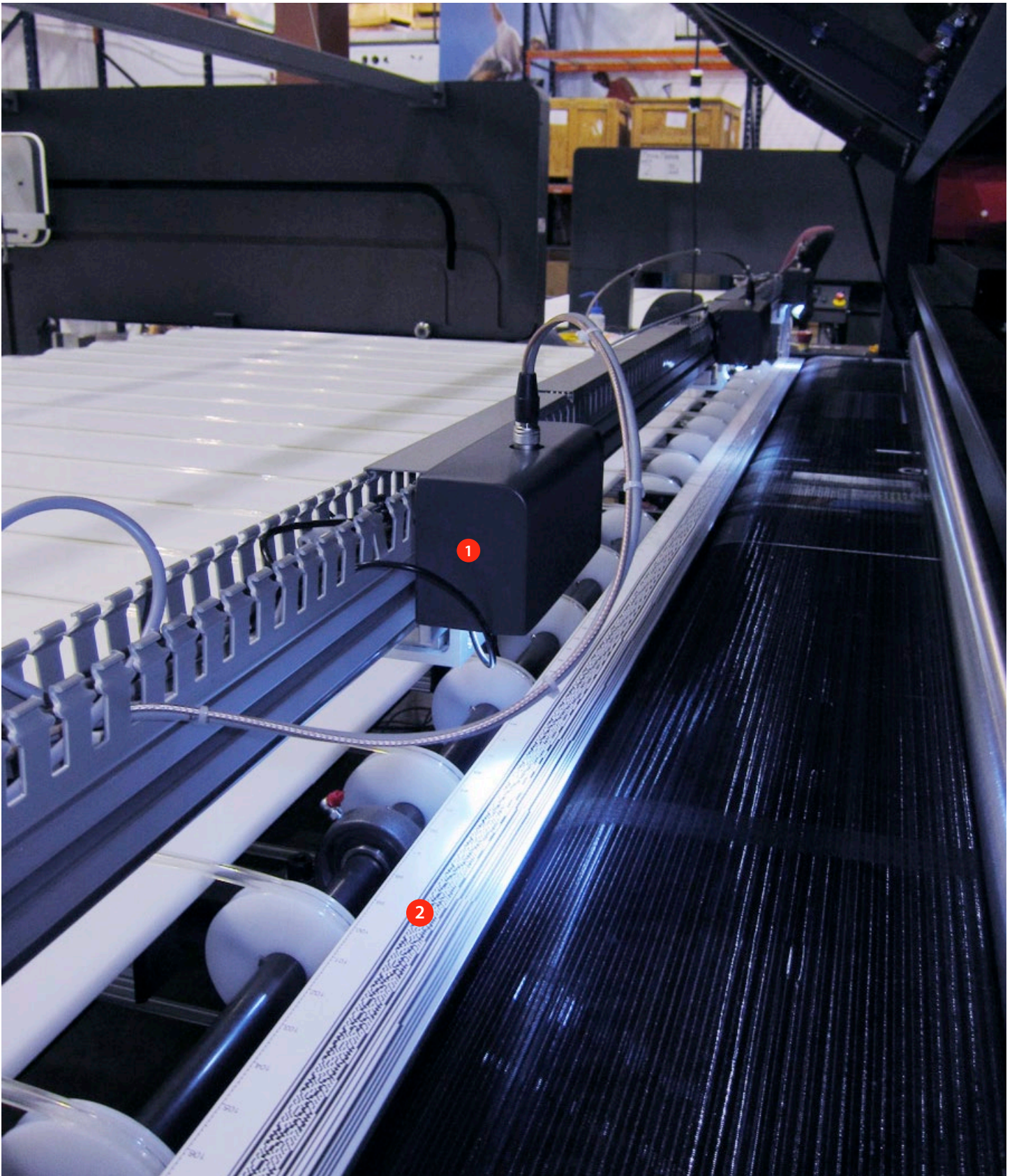
A camera (1) reads the position of each incoming board comparing the edge of the board against a registration code (2) printed in the edge of the rear table.
