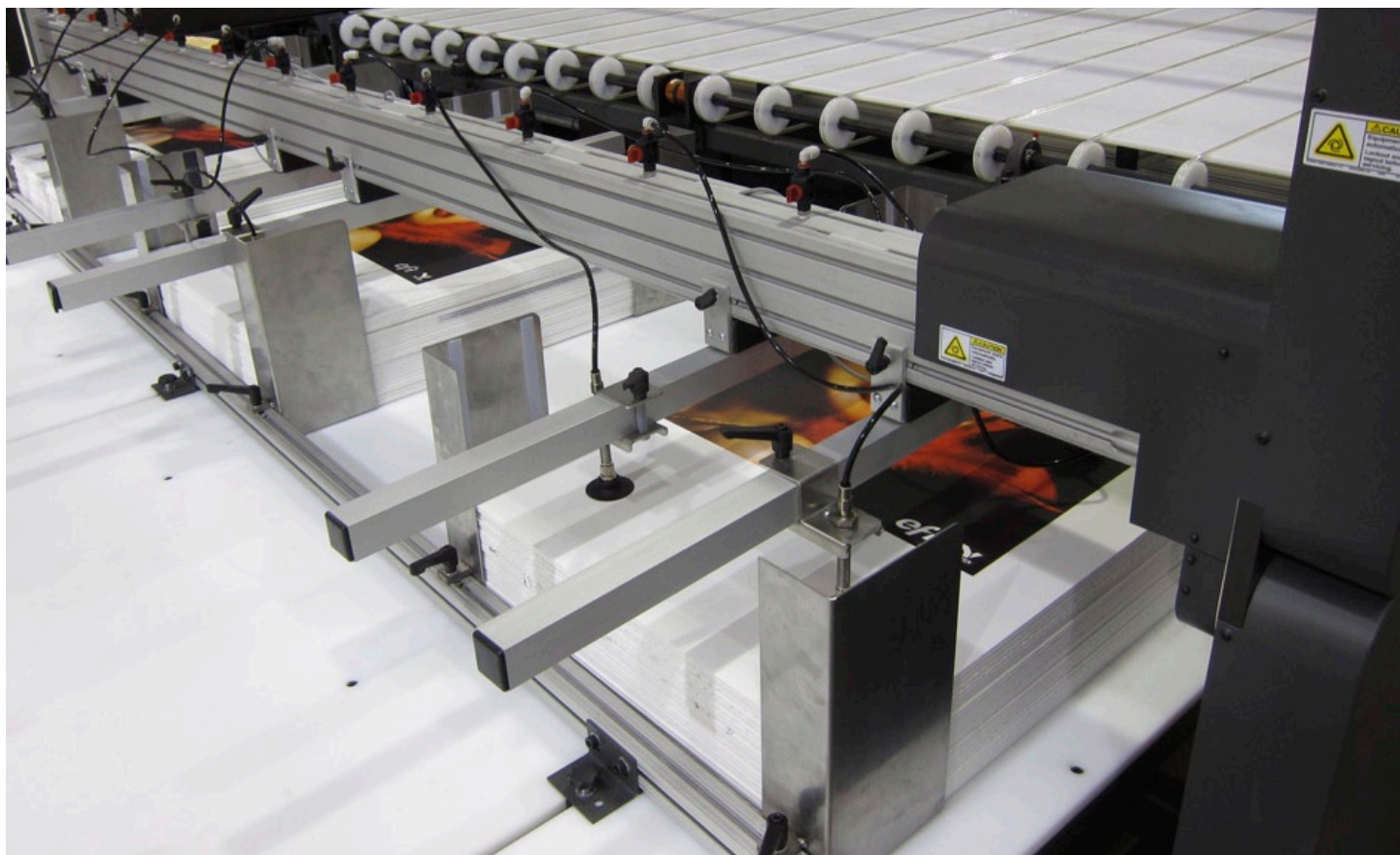
Similar pieces make it possible to stack the boards perfectly aligned at the front.
