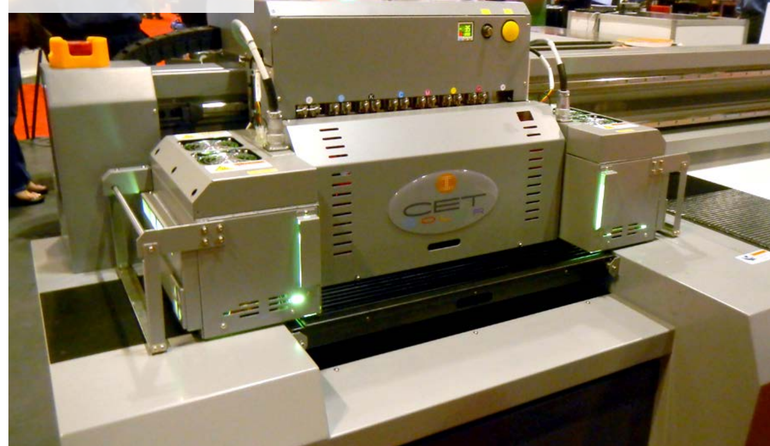
Close up, CET X500 UV printer carriage.
