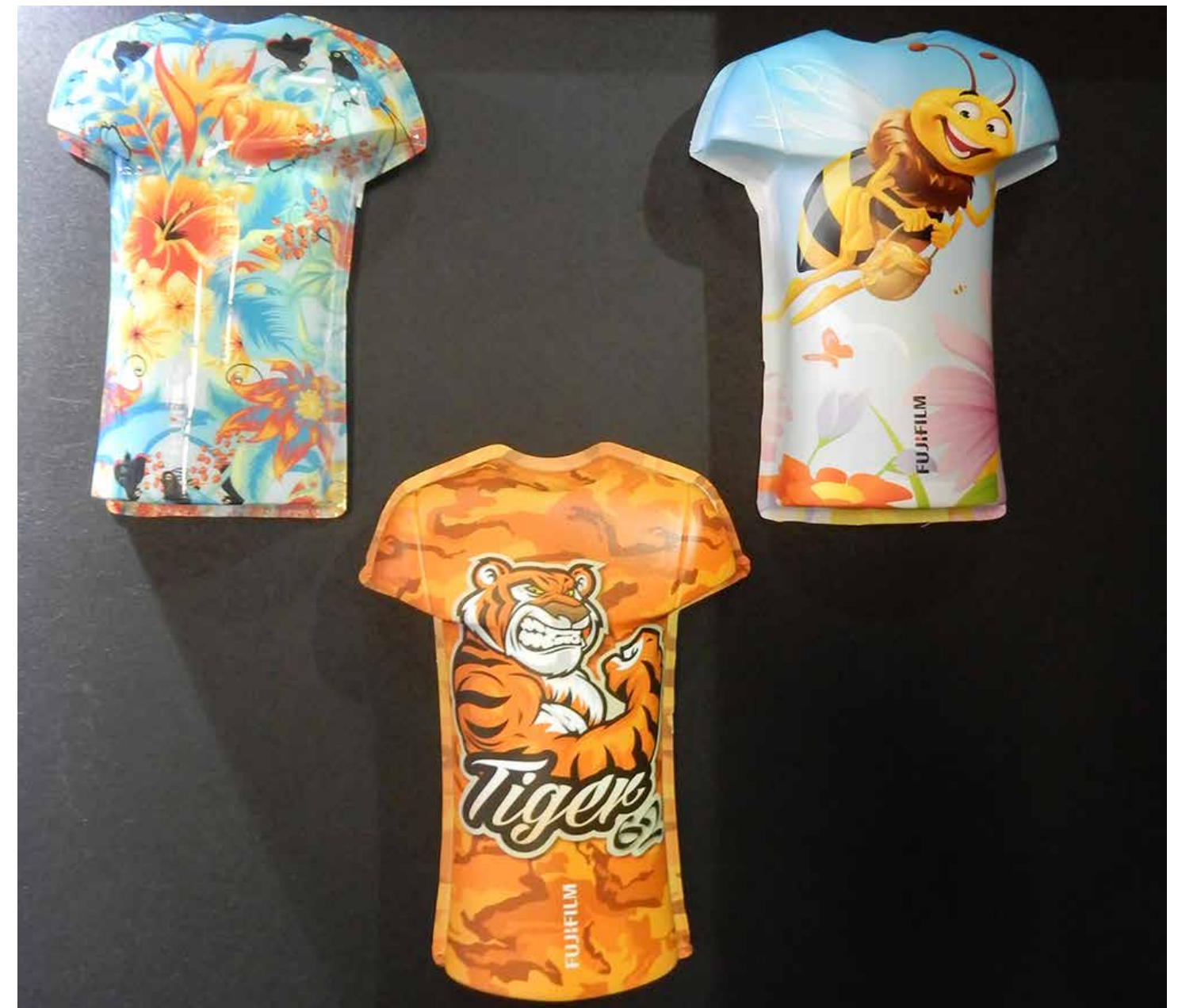
Fujifilm Acuity Advanced thermal vacuum formed sample. They had a full demo area: all the equipment to show everything, plus they were doing each step so you could see the entire process easily. Very nicely displayed with a patient and knowledgeable operator.
