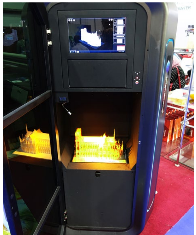
PrismaLab Rapid400, closet-sized 3D printer, Made in China (Shanghai). Booth of Sabazu (same booth as DOCAN UV-cured flatbed printer).
