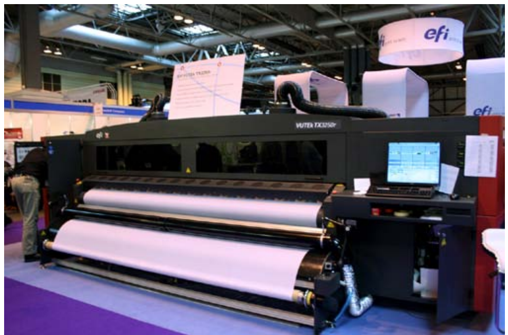
Here is the EFI VUTEk TX3250r printing some samples, as you can see at the photo you will need a calendaring machine to fixate the colors.
