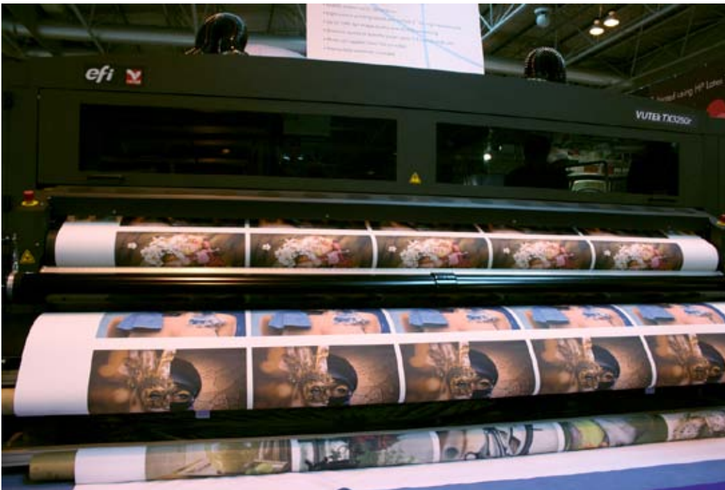
Here is the EFI VUTEk TX3250r printing some samples, as you can see at the photo you will need a calendaring machine to fixate the colors.
