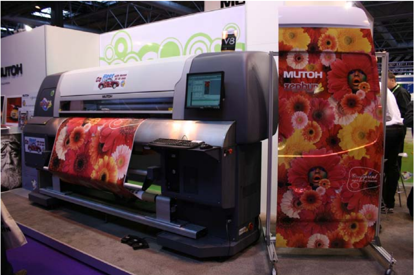
Mutoh Zephyr printing some samples with 3D inks, at the right we can see some wrapping sample printed with same inks.
