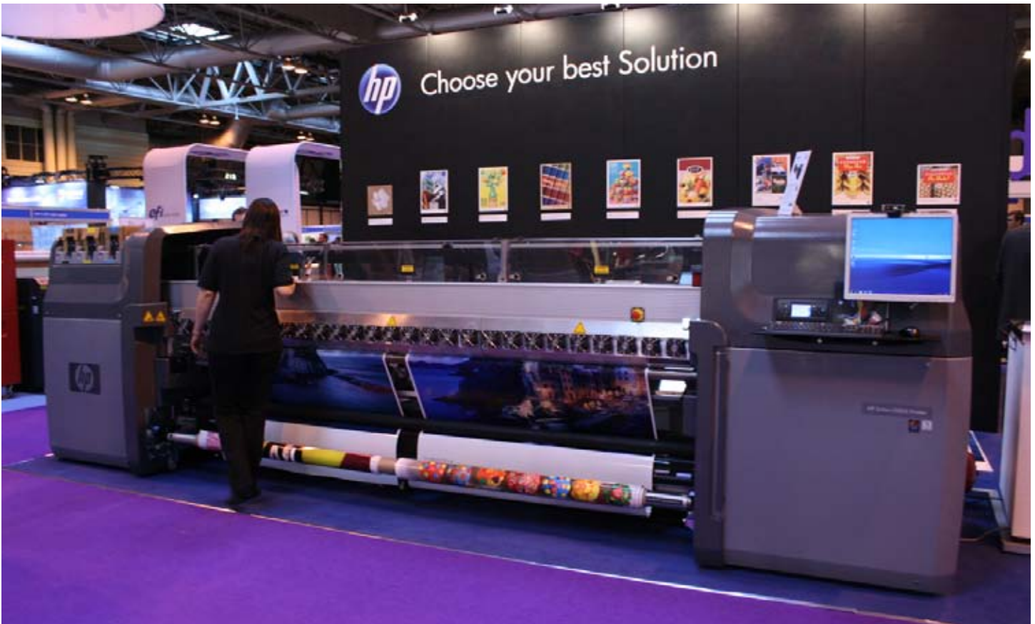
HP LX800 printing some samples at HP booth, you can print some textiles with this printer with extra accessories.
