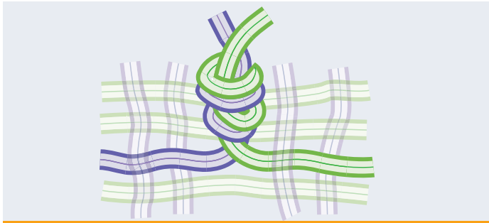
Knots in fabric, caused by two threads tied together.
