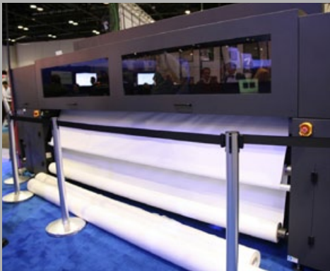
Rear view of the EFI R3225. As you can see in the diagram, media is loaded at the back.
